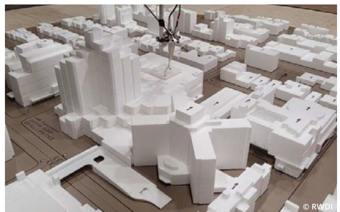
Figure 2: 1:300 Scale model of Vancouver General Hospital in RWDI's Davies Boundary Layer Wind Tunnel instrumented with Cobra probes to measure the mean and fluctuating wind speeds.
