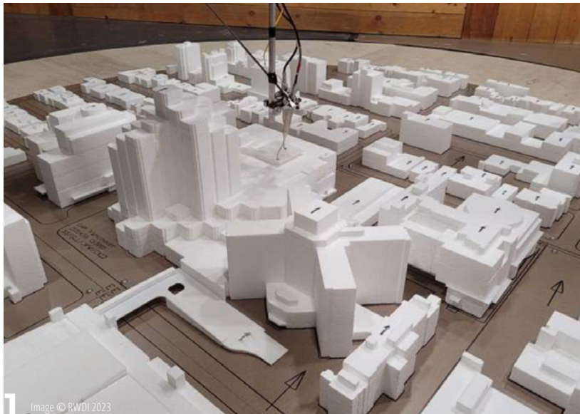
Figure 1: 1:300 Scale model of Vancouver General Hospital in RWDI's Davies Boundary Layer Wind Tunnel instrumented with Cobra probes to measure the mean and fluctuating wind speed above an existing heliport.
