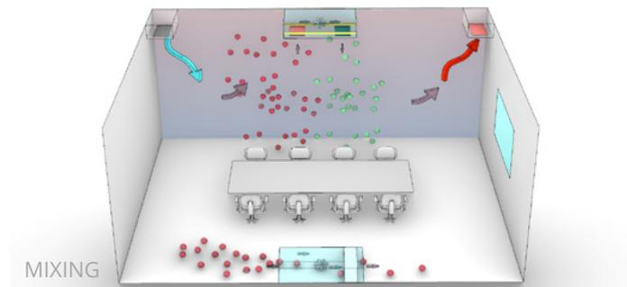
*A mixing ventilation system can benefit from both in-room filtration and upper-room UVGI.*
