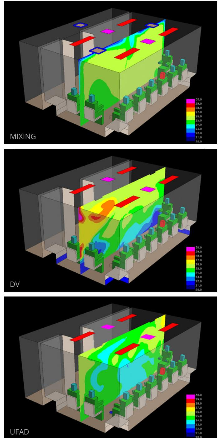
Figure 1 - Temperature distribution in a meeting/waiting room for three different air-distribution methods
