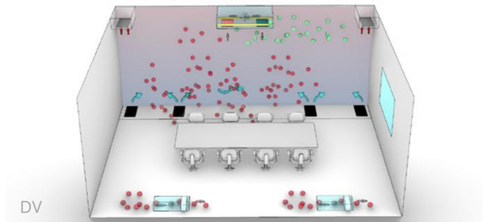
*For displacement ventilation, neither upper-room UVGI or in-room filtration can help. The clean particles from the UVGI will leave the room at the ceiling and the in-room filtration runs the risk of breaking up the stratification layer.*
