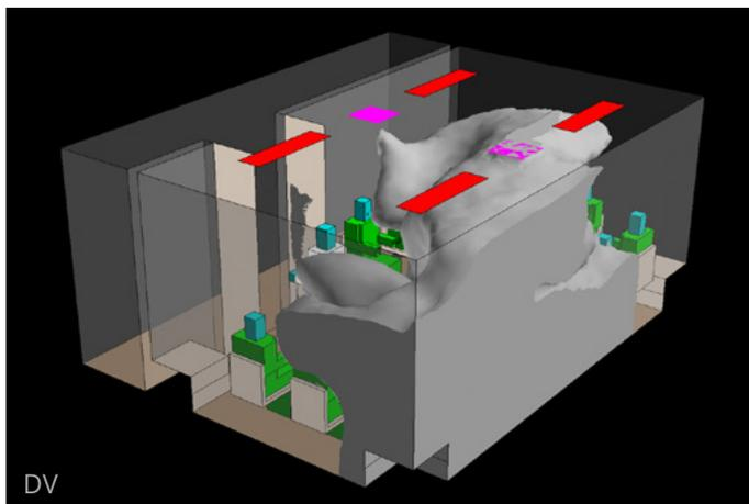
On the other hand, the **displacement ventilation system** is doing its job. The blue surfaces are introducing the air with minimal mixing and the contaminants are being lifted to the ceiling by the thermal plume around the ill occupant. The rest of the room is clear.
