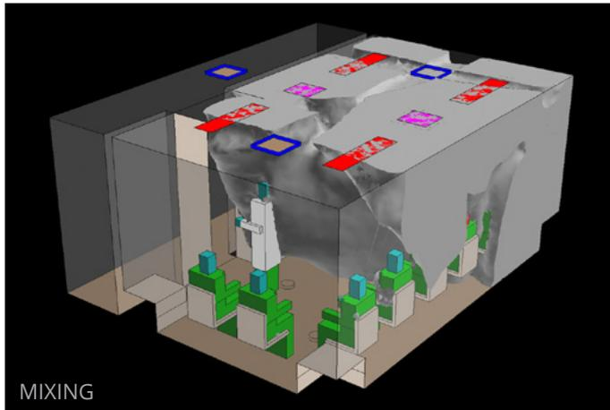
The **mixing system** is mixing the droplets around the space as rapidly as possible. The reason that the foreground in the image is not completely greyed out is because the ceiling supply air diffuser at the front of the image is diluting the contaminant in that zone—the ill occupant is at the other end of the room. If we selected a dilution of 1/1000 to present (100 droplets per breath), then it is likely that the cloud would expand and fill the room.
