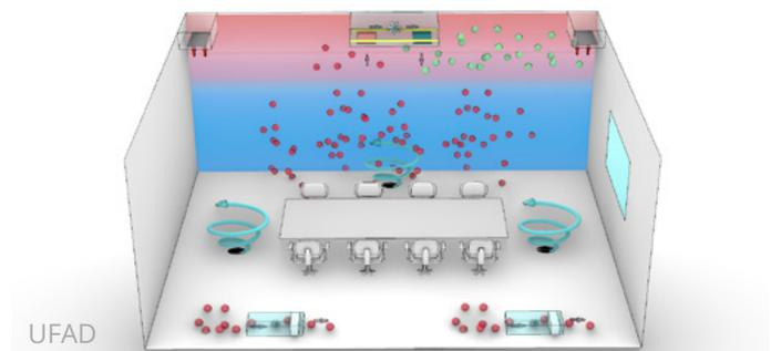
*A UFAD system is not supported by the use of upper-room UVGI as the clean particles will leave. A distributed in-room filtration can help provided it does not break the stratification layer.*
