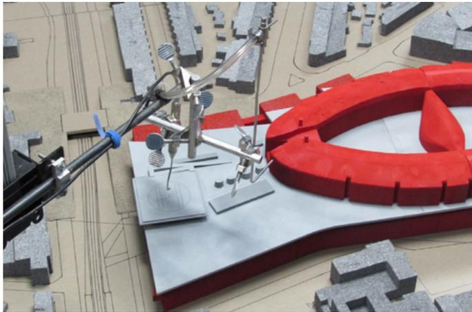
Figure 1: Model of New Children’s Hospital Helipad, Dublin Ireland being tested in RWDI’s wind tunnel. Model is instrumented with Cobra probes to establish turbulence conditions near the helipad.
