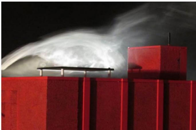
Figure 2. Building structures nearby can create problematic turbulence at the vertipad. Here in an image from a wind tunnel test, the wind is coming from the left. While some of the airflow passes over the small structure on the right, most of it curls under to produce a region of turbulence directly over the vertipad which is not good.
