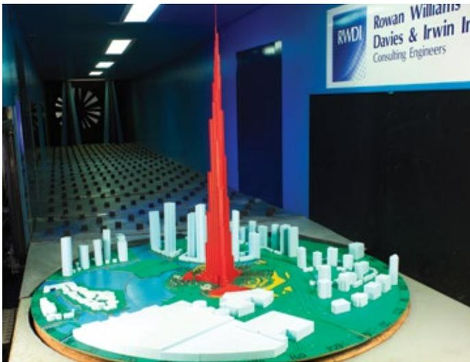
Figure 2. Burj Khalifa wind tunnel model. Stepped setbacks into the building were introduced, and the base was rotated to improve its aerodynamic efficiency in the direction of strongest winds.
