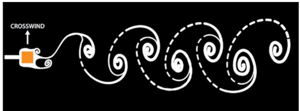
*Figure 1. Sketch showing vortex shedding flow patterns. These regularly spaced vortices generate their largest forces perpendicular to the direction of flow, causing crosswind vibrations.*
