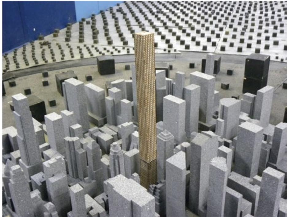
*Figure 5. Initial wind tunnel model of 432 Park Avenue that was tested before the exploration of openings in the shaping workshop.*
